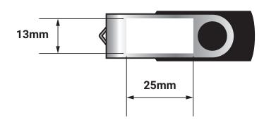
PRINTABLE AREAUSB DIMENSIONS25mm x 13mmL: 58mm x W: 10mm x H: 18.5mm
